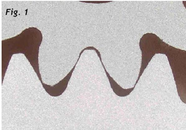
Direct Gear Design optimizes the gear tooth in the normal section, making it suitable for any kind of involute gears: spur, helical, bevel, worm, face, etc. It expands the current limits of the following involute gear parameters:
