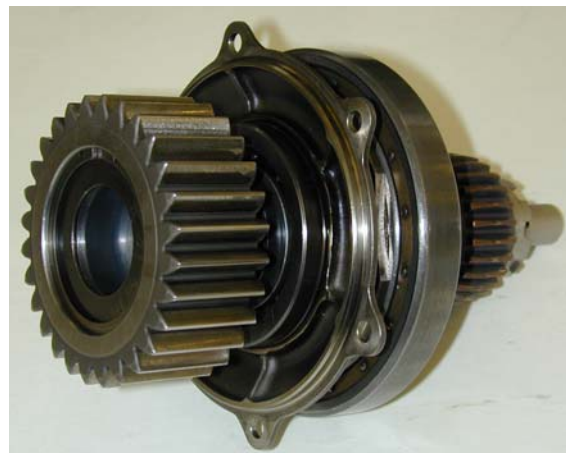
Fig 7. First stage sun gear assembly
