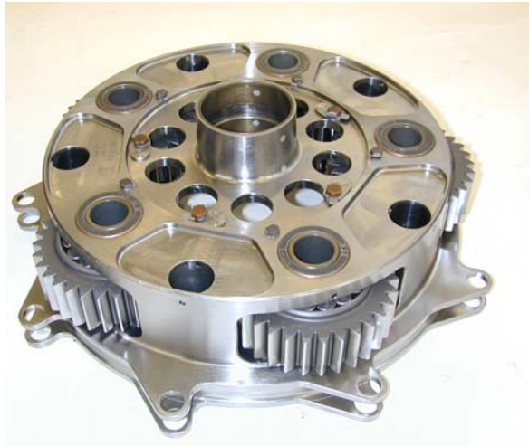
Fig 10. Second stage carrier assembly
