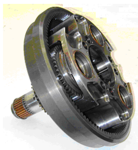
Fig 8. First stage carrier and ring gear assembly
