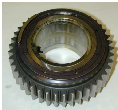
Fig 9. Second stage sun gear
