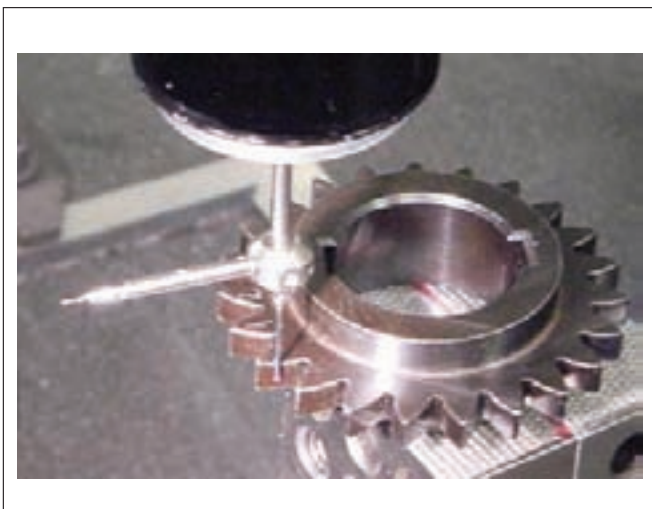
Figure 10—CMM measurement of asymmetric gear.
