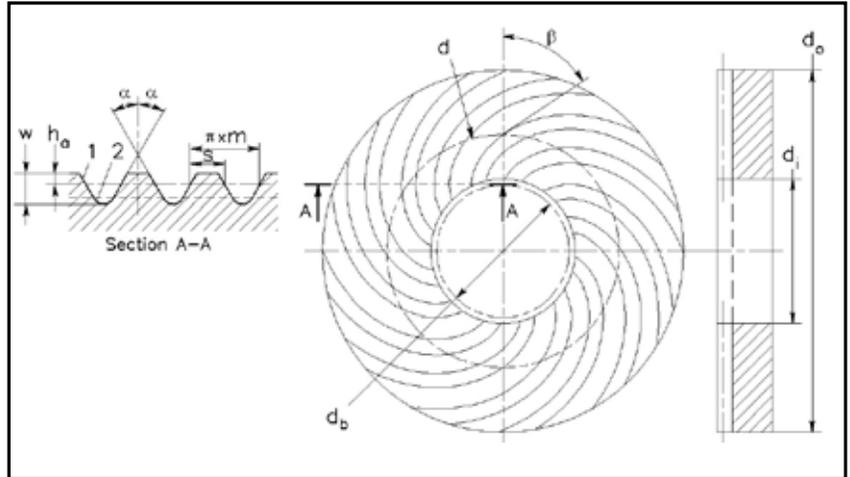
Figure 1: Face involute spiral gear;  $d_b$ ,  $d_i$ ,  $d$ , and  $d_o$  are base, minor, reference and major diameters,  $\beta$  is spiral angle at reference diameter,  $m$  – module,  $a$  – profile (pressure) angle,  $s$  – tooth thickness at reference (pitch) line,  $h_a$  – tooth addendum,  $w$  – whole depth; 1 – tooth flank, 2 – root fillet
