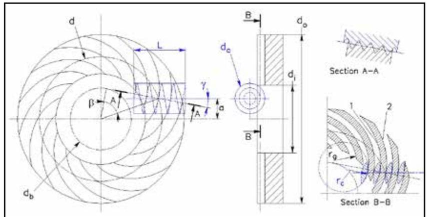
Figure 2: Schematics of left hand spiral face gear (black) hobbing with right hand hob (blue);  $\gamma$  – hob lead angle,  $L$  – hob length,  $d_c$  – hob major diameter; section A-A is tangent to base circle  $d_b$  and normal to the gear tooth line; section B-B is parallel to the hob axis, 1 – concave gear tooth flank, 2 – convex flank
