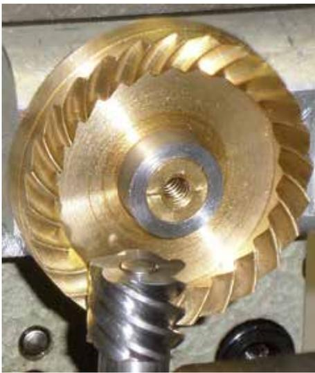
Figure 8: Sample of spiral face gear pair
