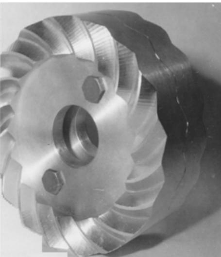
Figure 7: Sample of involute spiral face coupling assembly
